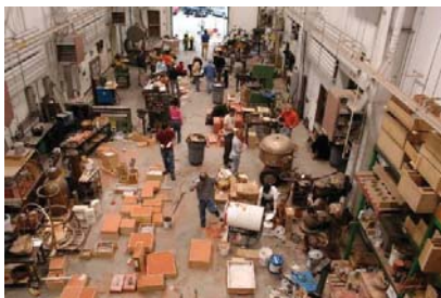
Preparing molds for iron pour in the sculpture foundry
